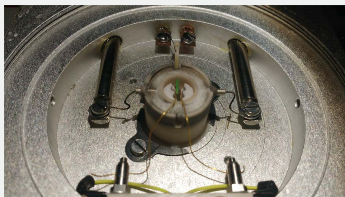
Figure 2. The mounting of the Ni-YSZ symmetric cell in the Linkam stage
