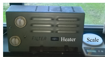
Figure 2.5: The heater applied for the water content test (left) and the scale (right).
