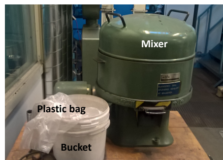
Figure 2.4: The mixer together with the bucket containing the homogeneously mixed green sand.
