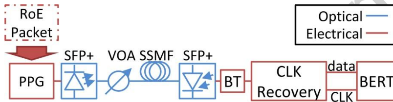
Fig. 7: RoE structure to evaluate bit error rate
