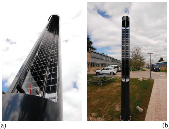
FIGURE 3. (a) The prototyping setup of the bifacial PV cell with its retroreflector as illustrated in Fig.1. (b) The prototype is mounted on ground level.
