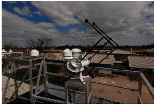
FIGURE 2. The tracking solar setup measures the normal incidence of light from the sun. The black sphere obstructs direct sunlight to a horizontal detector, which measures the diffuse light.
