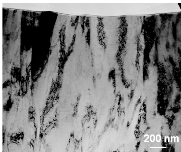
FIG 13 A cross-sectional BF micrograph showing flat multilayer fringes, smooth surface and completely void-free columnar structure in the TiAlN/VN (-125V).
