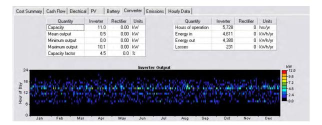
Fig. 3. Battery component annual simulation results for the homestead's input from the  $6 \text{ kW}_p$  PV and the output to the 11 kW<sub>p</sub> inverter.
