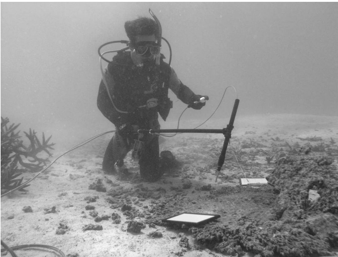
Figure 4-1: The underwater spectrometer setup for collecting spectral reflectance signatures of habitat components in shallow water. Note the remote trigger held in the diver's left hand and the Teflon reflectance panel in the foreground. Note that this image was not taken at Rottnest Island.
