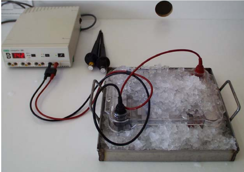
Figure 3-2. Photograph of horizontal gel bed packed in ice and used for the IRS-PCR method
