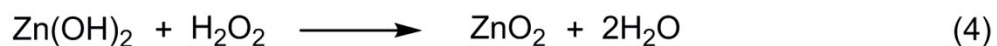
Figure 2.2.1: Reaction mechanism for the synthesis of zinc peroxide nanoparticles via the precipitation method.
