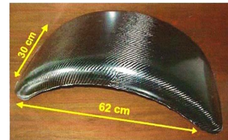
FIG 4. X-ray cured six-ply carbon fiber composite motorcycle fender.
