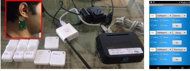
Fig. 6. (a) PogoPlug Smart Home Customized Devices (from left) PIR sensors, object sensors, Ethernet Tag Manager, PogoPlug Mobile, Simplelink SensorTag used in the neck (top left corner) (b) Base application
