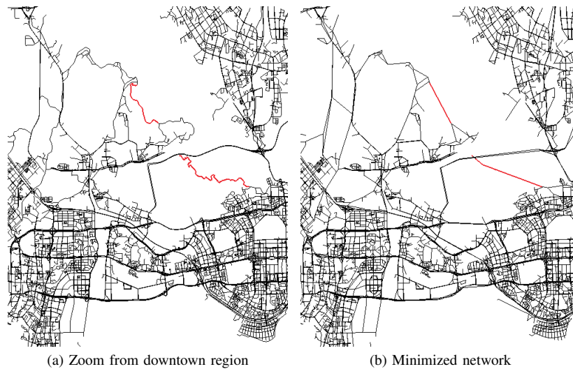
Fig. 5: Comparison between the original shapefiles and the minimized network. Two roads in which this difference is particularly notorious have been marked in red.
