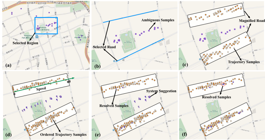
Fig. 7. Resolving ambiguities. (a) User selects a region to resolve ambiguous samples. (b) System suggests two candidate roads according to the directions of the ambiguous samples. (c) The system magnifies the candidate roads and shows the trajectory samples positioning on the roads. (d) Trajectory samples and ambiguous samples are sorted according to their speeds. And the system provides suggestions for the ambiguous samples. (e) User makes the decision according to the system suggestions. (f) Ambiguous samples are resolved and placed on the roads.
