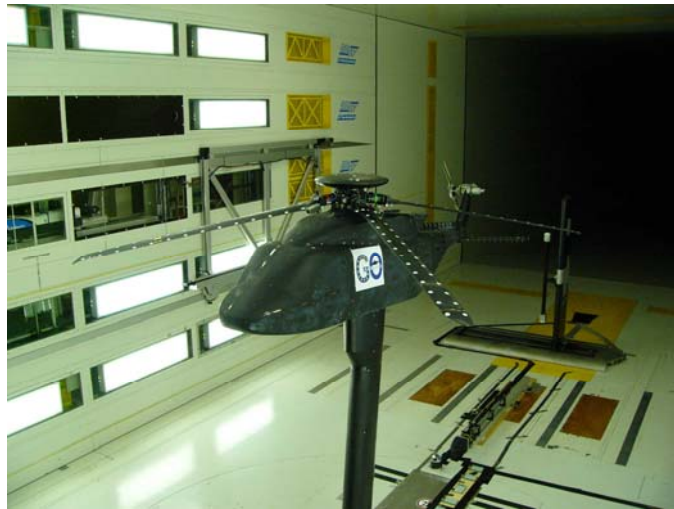
Figure 1: The GOAHEAD configuration inside the DNW-LLF wind tunnel
