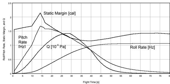
Figure 6. Ascent Flight Parameters
