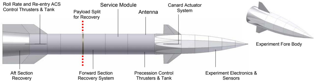
Figure 4. Main Payload Components
