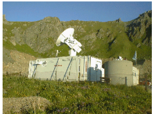
Figure 5. RIR-774C C-Band Tracking RADAR for range safety operations at Andøya Rocket Range, Norway
