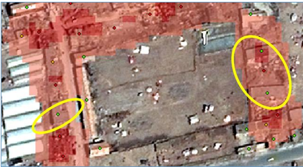
Figure 5.3: Distorted data representation caused by interpolation (here: KDE): red and yellow dots are damaged buildings, green points represent undamaged buildings. This effect is additionally enforced in densely populated areas
