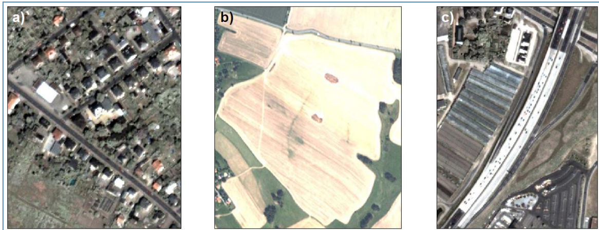
Figure 2.8: Problems with VHSR satellite data a) Lacking spectral discernment (similarity between roofs and streets), b) spectral variability of a single image object (different degrees of ripeness in a grain field), c) interfering image objects (cars on street).
