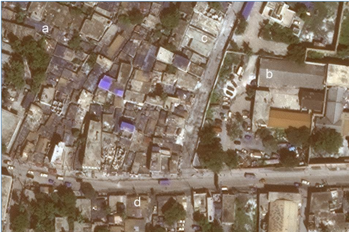
Figure 6.3: Illustrative examples of common problems for OBIA in the Haiti case: a) similar spectral values of roofs belonging to different houses b) shading of roof-parts belonging to the same dwelling c) low differences in spectral reflectance between buildings and streets d) spectral similarity of roofs and backyards
