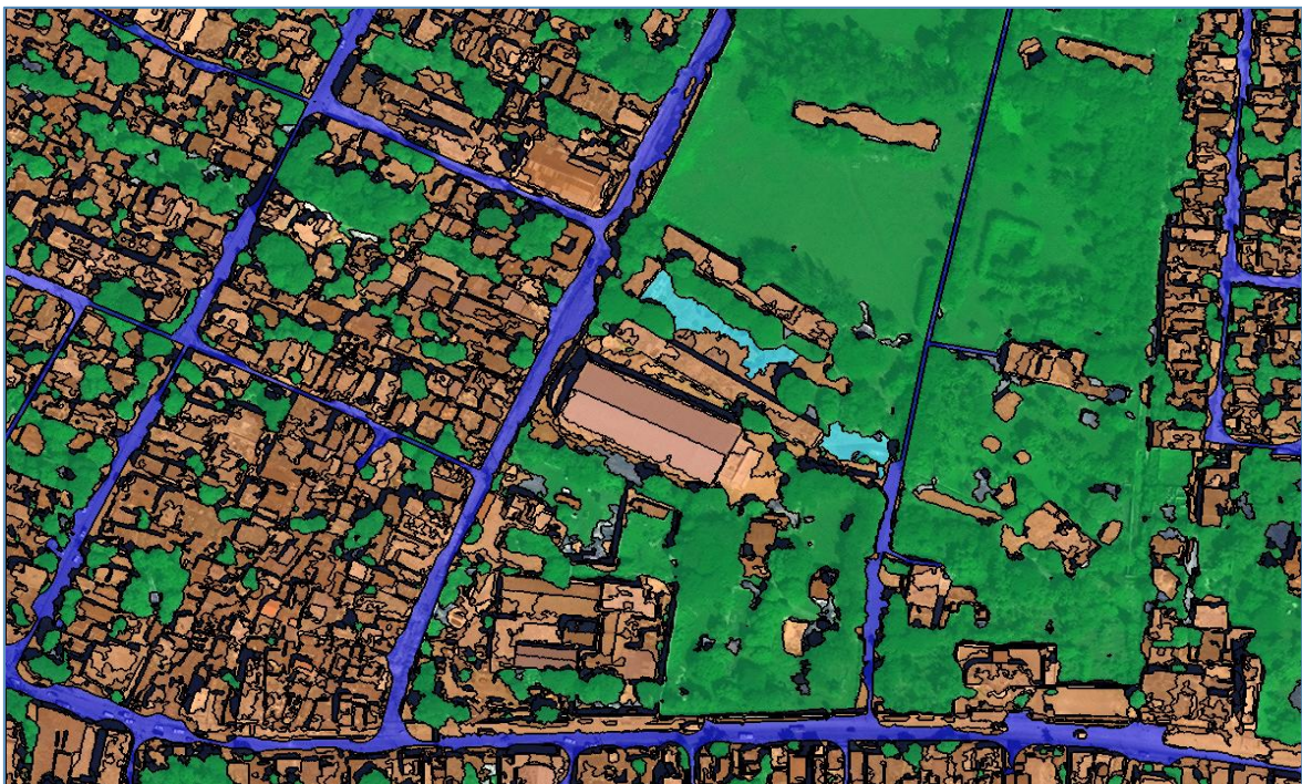
Figure 6.2: Classification example of a GeoEye-1 subset in Carrefour, Haiti (blue: streets; green: vegetation; light-blue: sealed soil; orange: built up areas). The house in the centre of the image shows an example of over-segmentation
