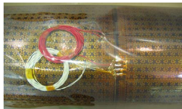
(b) Implemented electric heater applied to a rigidizable inflatable boom by Alcatel Space (extracted from [8])
