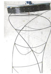
(b) Very light SAILMAST by ATK (extracted from [46])
