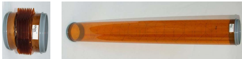
(a) Packed (left) and deployed (right) inflatable tubular boom by EADS-ST [13]
