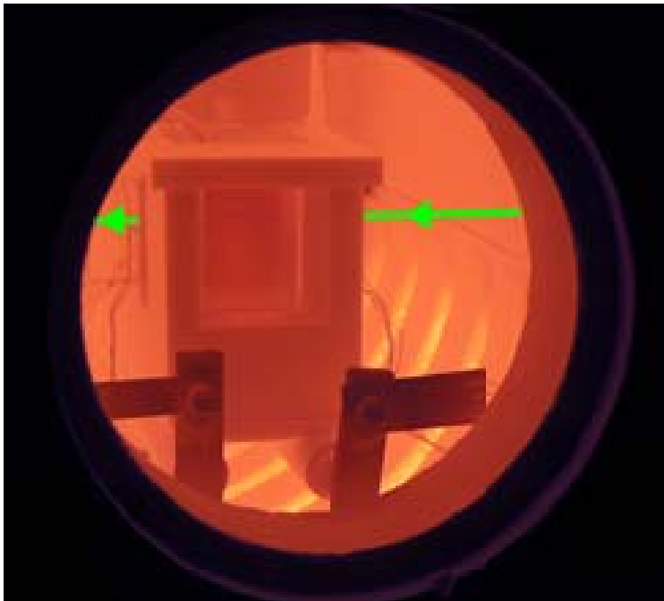
Fig. 4: Photo of the SOFC cell compartment through the observation window for the detection of the Raman scattered radiation. The furnace is at T \approx 1123 K. The central part is the transparent flow field consisting of quartz glass and surrounded by ceramic parts. The green line indicates the laser beam.
