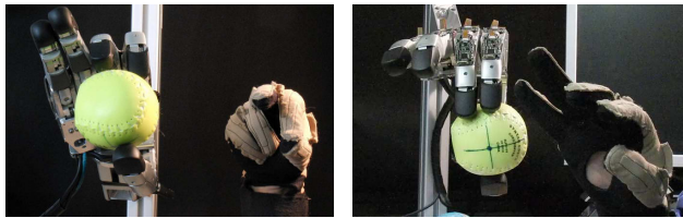
(a) Task space telemanipulation. (b) Joint space telemanipulation.
