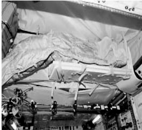
Figure 6: Polyethylene panels installed in the crew sleeping quarters of ISS. Picture from NASA, Office of Biological and Physical Research.
