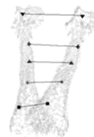
Fig. 8 Translational discrepancy is defined as the mean distance between surface points. Here five example points are shown.
