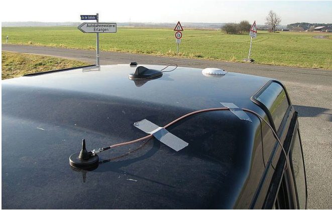
Fig. 7 Picture of mobile measurement setup (front: monitoring antenna for transmit spectrum; center: Fraunhofer S-band transmit antenna; white: DVB-SH receiver antenna; left, back: GPS receiver)
