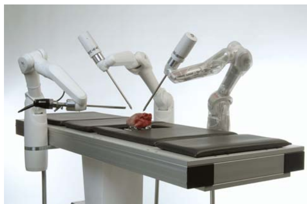
Fig. 2 The DLR MiroSurge robotic system
