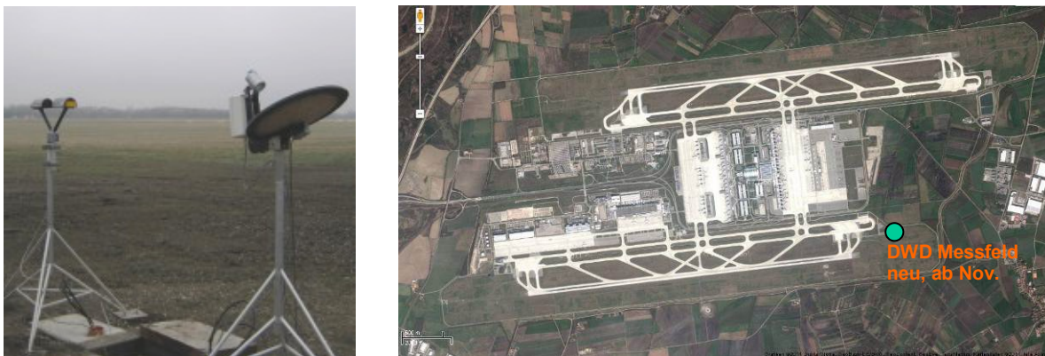
Figure 3. Observation instruments at Munich airport operated by DLR, foto: Parsivel (left), micro-rain radar (right), observation site indicated by green dot in right Figure.
