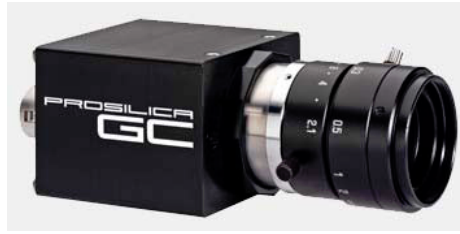
Figure 9. Prosilica GC-655 used as optical sensor in rendezvous simulations
