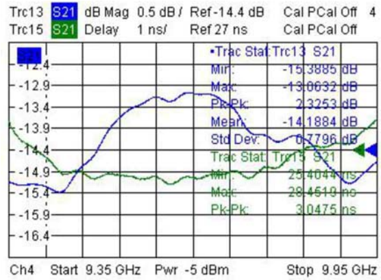
Figure 4 Magnitude and group delay of the transfer function of the whole transponder chain measured with a network analyzer (additional 30 dB attenuation at the input, 50 dB at the output).
