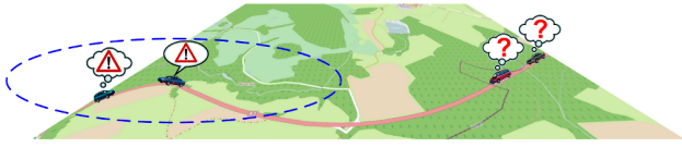
Fig. 2. Clustering of VANETs in case of low density of equipped vehicles. Information dissemination is possible only between vehicles within the same cluster (left), but not between different clusters (from left to right) without any additional mechanisms.
