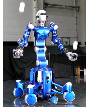
Fig. 1. Rollin’ Justin [6] catching two simultaneously thrown balls. The mobile humanoid consists of an omnidirectional platform with variable footprint and an upper body with 19 active DOF, built from two DLR-LWR-III arms [7] with 7 DOF, a torso with 3 (+1 passive) DOF and a neck with 2 DOF, and is equipped with two 12 DOF DLR-Hand-II [8]. The system operates completely wirelessly using only onboard sensing (see Sec. V). Weight: upper body 45 kg; mobile base 150 kg.
