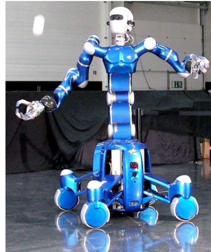
Fig. 8. DLR’s Rollin’ Justin catching a ball. For robust catching, the necessary accuracy is about 2cm in space and 5ms in time.
