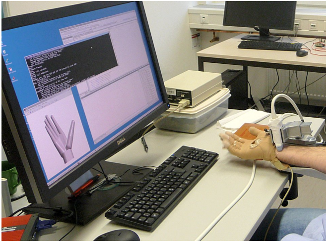
Fig. 2. The experimental setup: the subject would mimick the hand-model movements, as seen on the computer screen; meanwhile, the glove and ultrasound machine would gather hand motions and US images.
