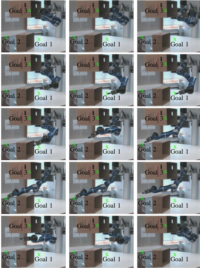
Fig. 5. Real-time motion planning at 500 Hz for a global 3-goals motion planning problem.
