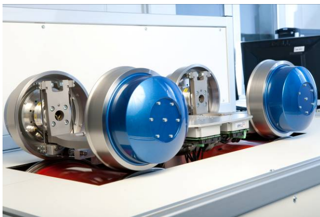
Fig. 4: Scaled 1:5 bogie on roller rig
