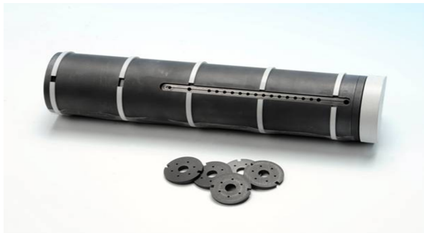
Figure 2. Newly designed high temperature shear-cell. The graphite articulation tube with lead-through for holding bolts is shown. The front part shows individual shear discs as they are integrated in the shear-cell. Cut-outs for disc motion as well as holes for diffusion samples are visible.
