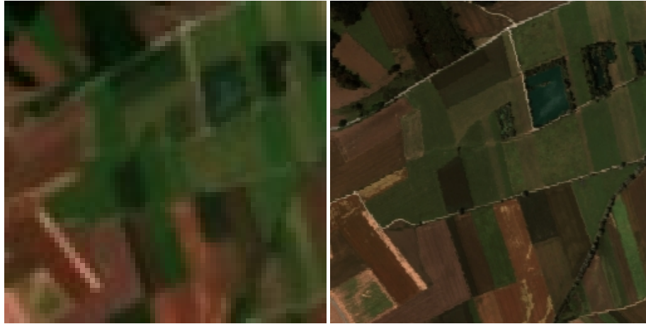
(a) 64 \times 64 pixels HyMAP hyperspectral input image. Image resampled from original image c). RGB composition, channels: 15, 7, 3. (b) Simulated, 256 \times 256 pixel Multispectral input image. Image resampled from original hyperspectral image c). RGB composition, channels: 5, 3, 2.
