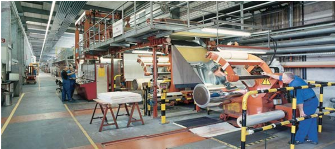
Fig. 6: Conveyer line for anodic oxidation treatment
