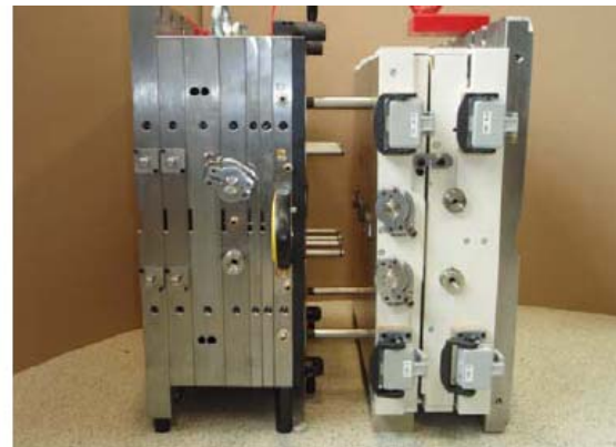
Fig. 4c/d: stack sealing design for FAST GDL sealing and in-mould assembly
