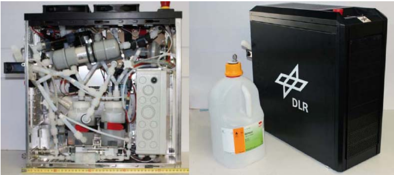
Fig. 8: DMFC portable stand alone system with open case and in PC enclosure
