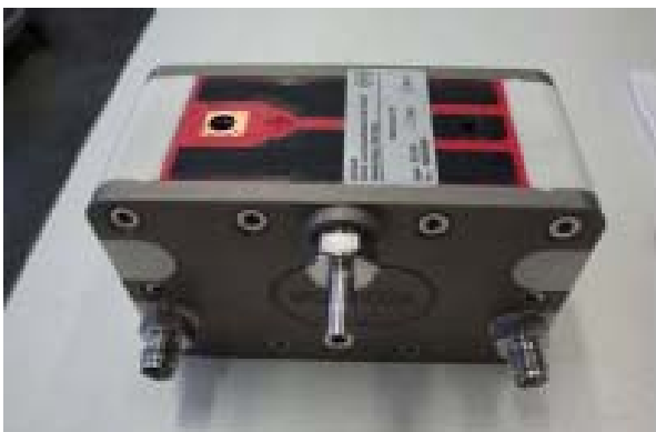
Fig. 6: short and full stack with lamination sealing concept
