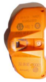
Fig. 7: Typical TPMS sensor mounted inside a tire
