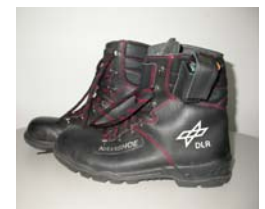
IMU: XSens MTx-28A53G25 foot-mounted: right and left
