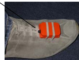
IMU: XSens MTx-28A53G25 foot-mounted: right and left
