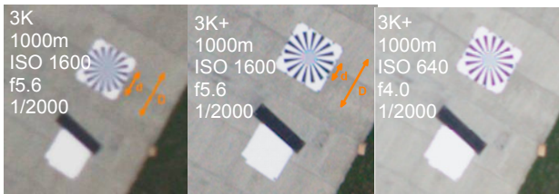
Figure 8: 3K and 3K+ images from a Siemens-star with fixed exposure time and variable aperture and ISO film speed.
