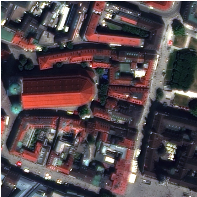
Figure 3. Pan-sharpened multispectral WorldView-2 image (bands:5, 3, 2) using GFF spectral fusion method.
