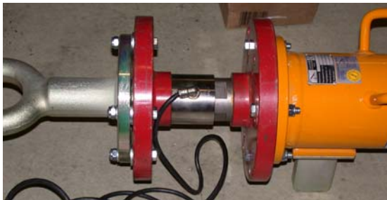
Figure 1: Towing force measurement with a load cell mounted in a towbar
