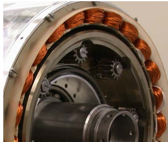
Fig. 9: View to the rotor with the rim-side planetary gears
