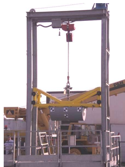
Figure 5 CIRA's LISA drop test facility
