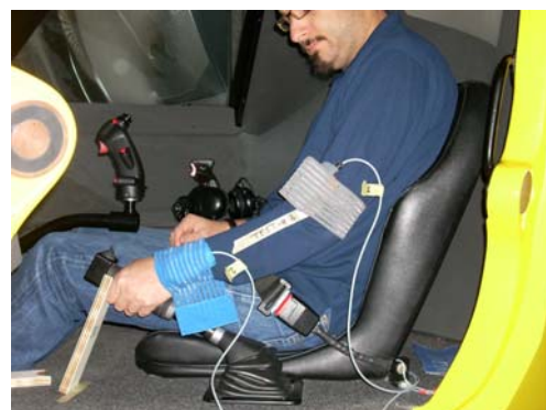
Figure 9 Test campaign in motion base flight test simulator (Univ. of Liverpool), biodynamic test campaign featuring pilot sensors
