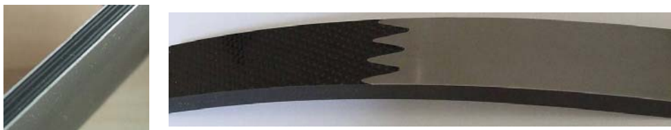
Fig 2.4: Skin protection with outer metal sheets (left). Abrasion protection (right). (Source:DLR)
