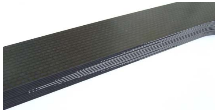
Fig 2.2: Transition region between CFRP and CFRP/steel hybrid material (source: DLR)
