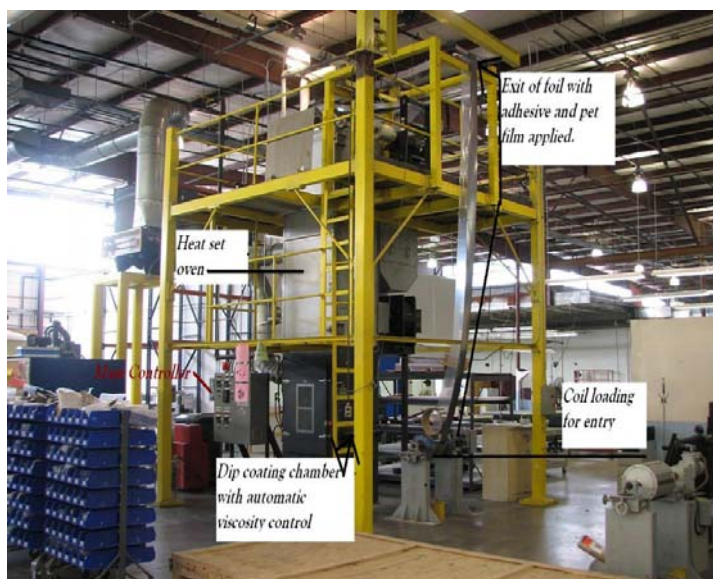
Fig. 3.6: MOD-3: Adhesive application.
