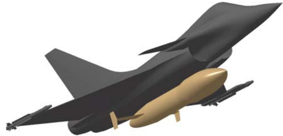
Figure 1: Experimental micro-launcher AML-X under belly of Rafale fighter aircraft
