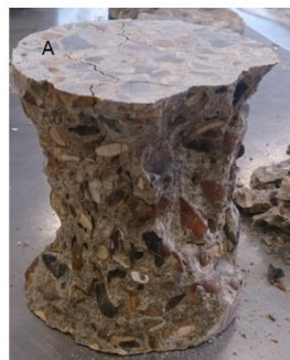
Figure 1, Satisfactory compression failure.
