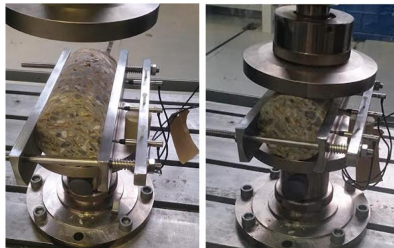
Figure 4, Core samples subjected to splitting test.
