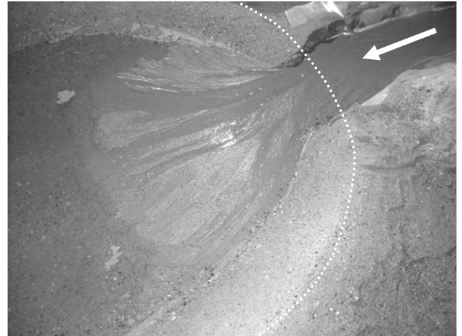
Figure 4. Numerous small incisions on the delta within the crater basin, with hardly any visible terraces. Flow is from top right to bottom left. D_{50} was 0.4 mm and discharge was 0.07 \text{ m}^3/\text{s} . Flow direction indicated by white arrow, crater rim outlined with white dotted line.
