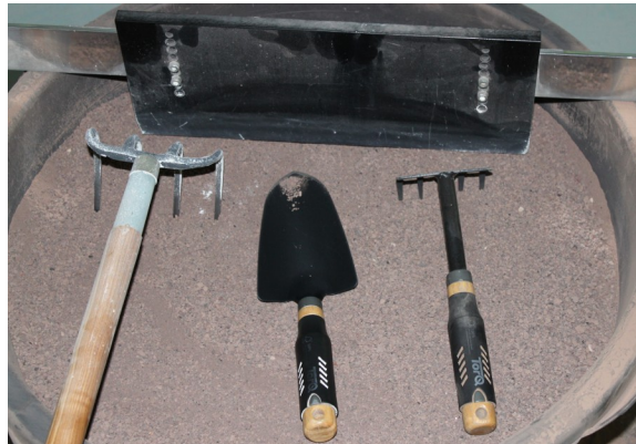
Figure 3: Tools used for soil preparation method testing; leveling board (above), garden rake (left), hand shovel (middle) and little hand rake (right)
