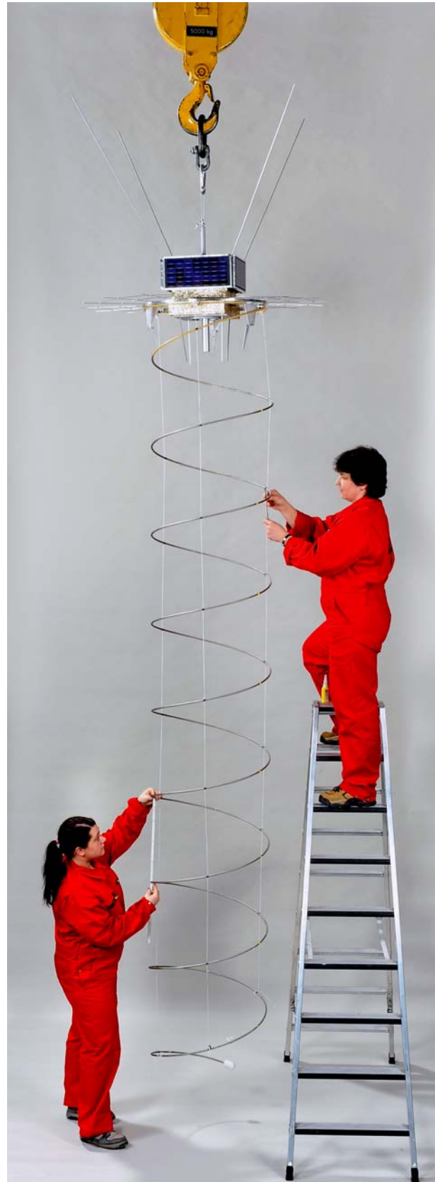
Fig. 2: AISat breadboard model with deployed antenna
