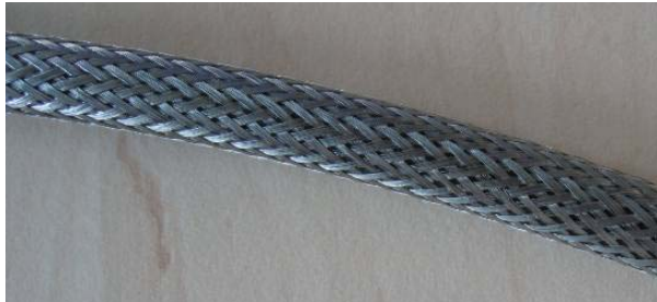
Fig. 8: Detailed view of the conductive coating. The tested antenna core diameters were 7 and 8 mm
