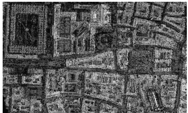
Figure 5. Disparity map with occlusions (black), section 1030 m × 630 m from the previously introduced Munich scene
