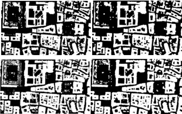
Figure 12. Derived building masks. Top row based on segmented disparity map, bottom row: filled original disparity map, left top/bottom: calculated map, right top/bottom: after closing and opening operations
