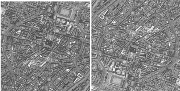
Figure 2. Section 2000 m × 2000 m from the Munich scene showing the center of the city, left and right stereo image
